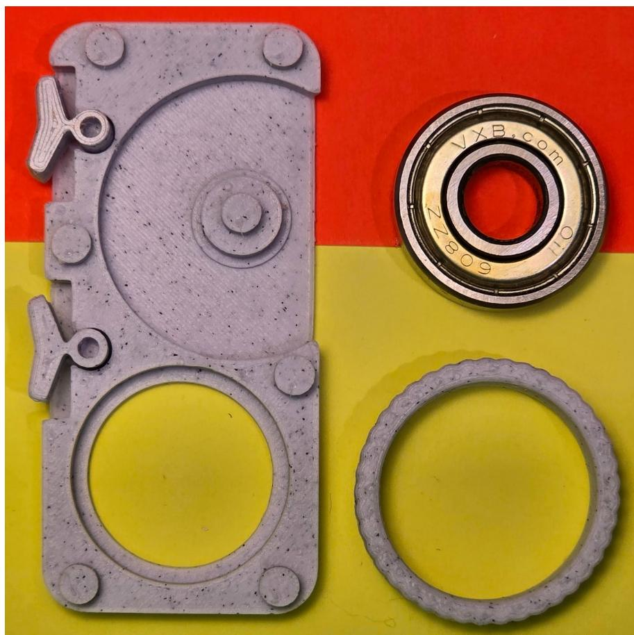
4- Put the **bearing** into the **ring**
