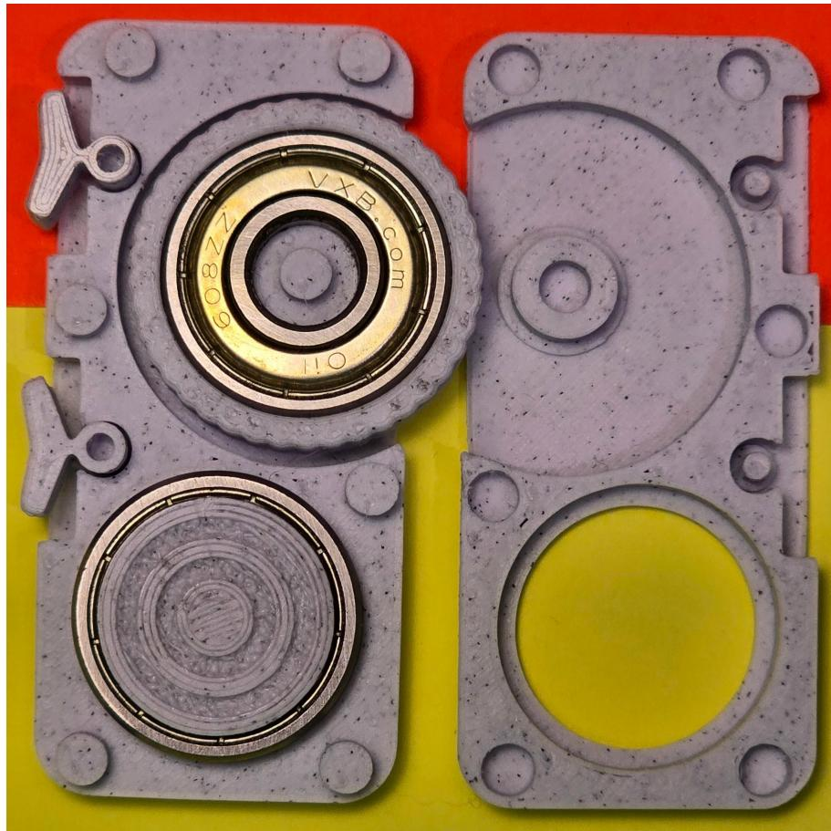
11- Put both **main sections** together. TIP: Take two flat surfaces and push them down so that both of the **main sections** go together without bending
